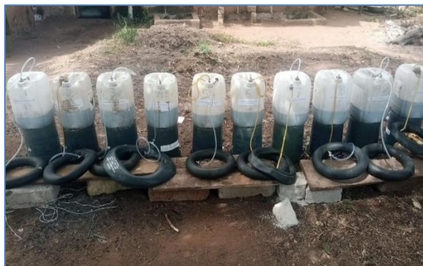
Fig. 1: Anaerobic digestion set-up outside the lab
